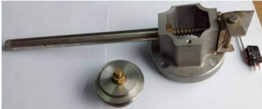
Figure 13) High-pressure pressure relief explosion-proof device
