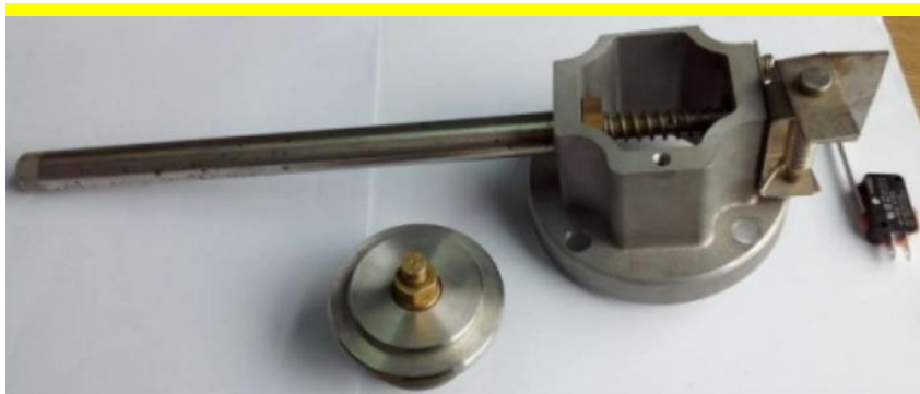
Figure 12) Low Air Pressure Lockout Indicating Device
